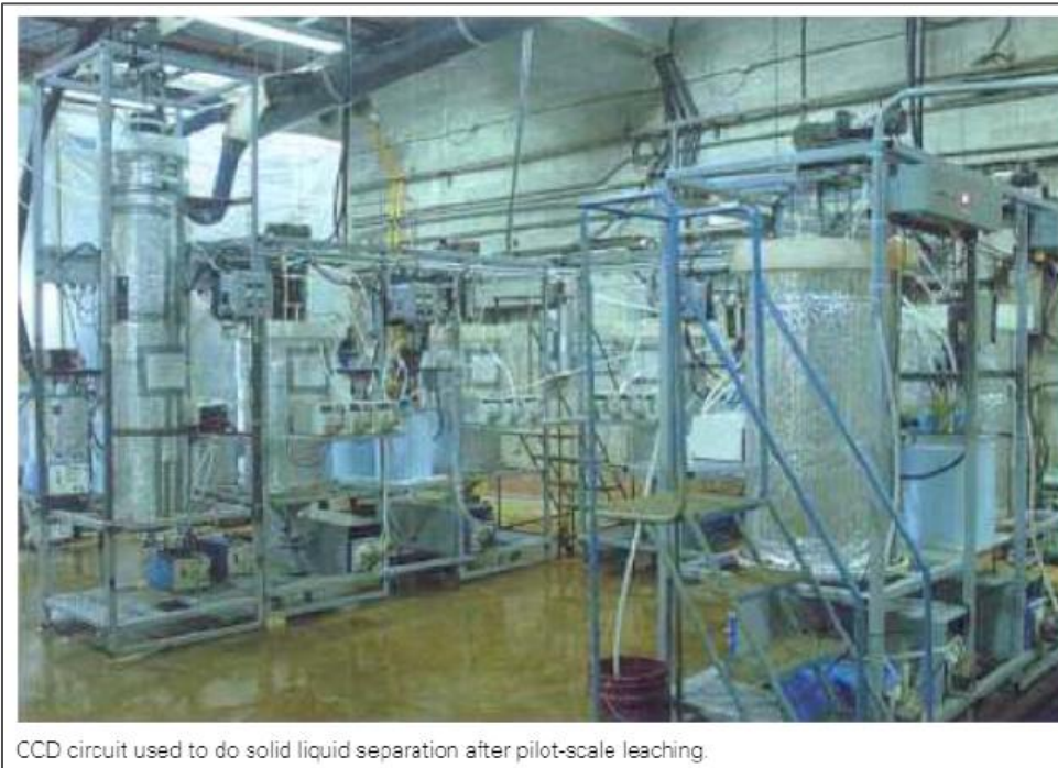
CCD circuit used to do solid liquid separation after pilot-scale leaching.
